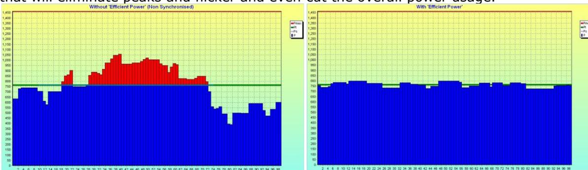
By using the PLM function, manufacturers are now able to use zero cross firing for their system without any drawbacks. Eliminating Phase Angle firing significantly improves the power factor which in turn results in substantial savings.
